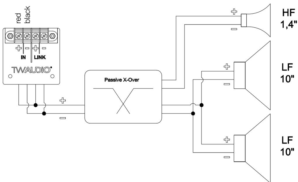
Figure 3.2 - Connection diagram
