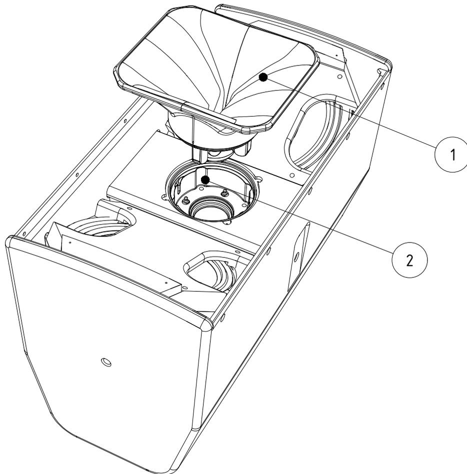
Figure 2.2.2 - setup of the T20i HF unit
