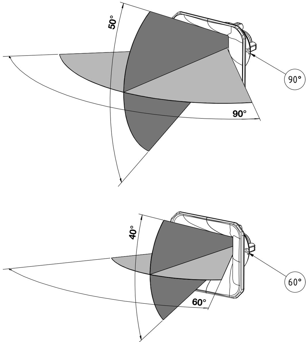
Figure 2.2.1 - Variants of the T20i HF horns
